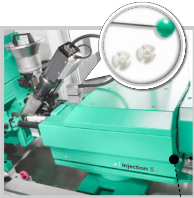
Micro-injection molding: extremely small shot weights thanks to the 0.1 oz micro-injection unit.
