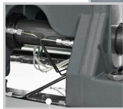
Maintenance-friendly: automatic central oil lubrication of the clamping unit.
