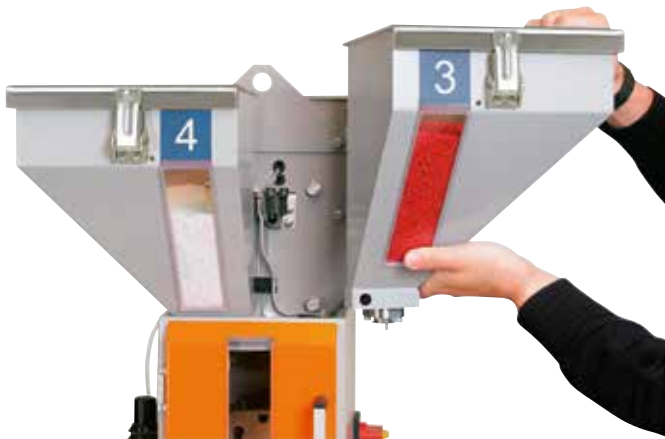
GRAVICOLOR 30 MD with removable supply hopper
