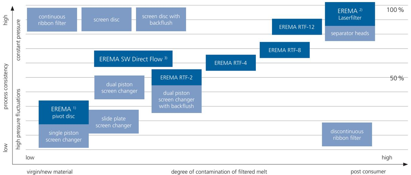
1) The **EREMA pivot disc** is suitable as safety filtration for clean polymer melts. Systems available: CL 104 (85 cm<sup>2</sup> active screen area), CL 120 (113 cm<sup>2</sup> active screen area)
