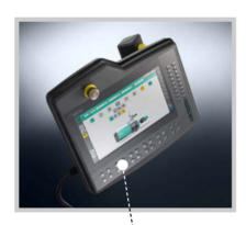
Mobile control system (optional): can be used universally for several machines and robotic systems.
