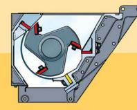
For more thick-walled and compact parts the Tangential cutter house is ideal. Standard configuration includes two fixed knives (red), if increased throughput is required, a third fixed knife can be specified (yellow).
