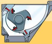
The Super-Tangential cutterhouse is ideal for voluminous parts and scrap providing excellent grip. Standard configuration includes two fixed knives.
