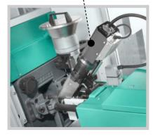
Flexible: the micro injection module can be easily replaced with a standard cylinder module.
