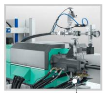
Process reliability: the cylinder module with liquid temperature control helps prevent premature cross-linking.
