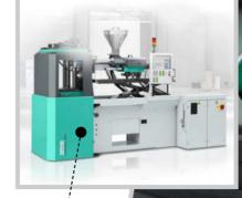
Electric mold height adjustment: the basis for high-speed, energy-saving cycles for 630-920 S machines. ALLROUNDER principle (optional): pivoting clamping unit offers even greater diversity in applications.
