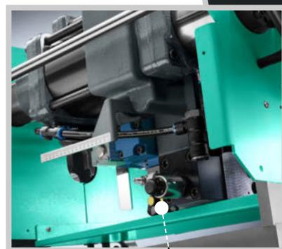
Precise: reproducible injection through valves situated close to consumers.
