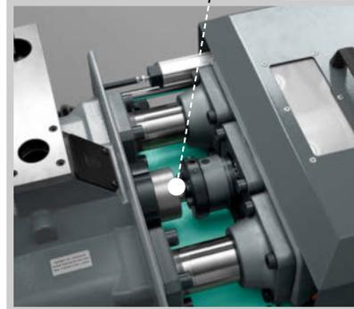
Swiveling injection unit: the screw can then be removed without dismantling the cylinder module.
