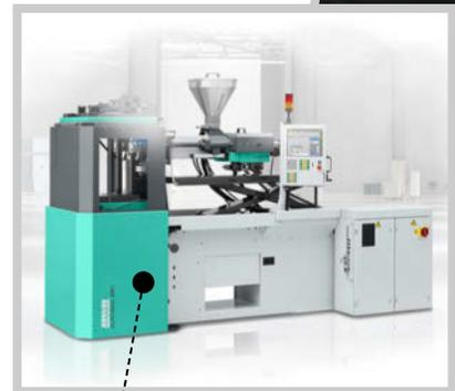
Simple conversion: quick-connect screw coupling and central coupling of all supply units of the cylinder module.
