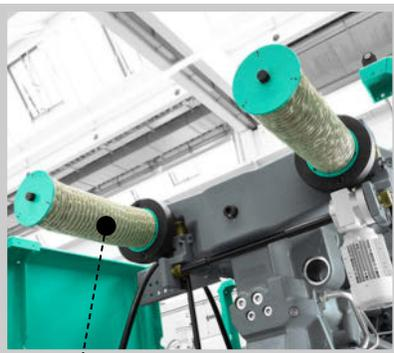
Electric mold height adjustment: the basis for high-speed, energy-saving cycles for 630-920 S machines.
