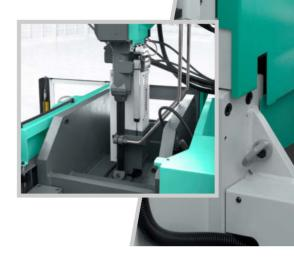
Simple conversion: central connection of all supply units of the cylinder module and screw rapid release coupling.
