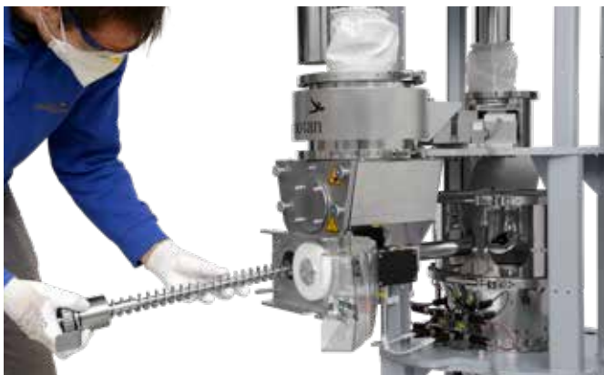
Easy exchange of dosing screws / gearboxes
