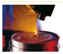
The centrepiece of the Laserfilter is the filter screen, which is where the name comes from. It features ultrafine boreholes which are lasered into the hardened special steel of the screen discs using extremely modern laser technology. A self-cleaning effect is achieved through the conical shape of the holes. Your quality bonus: the screen discs are made at EREMA's subsidiary 3 S.
